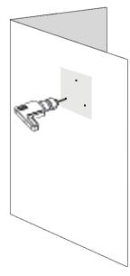
3. Use a drill to make mounting holes in suitable locations on the wall.
